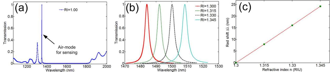
Fig. 2 (a) Transmission spectrum of the NPMC sensor from 3D-FDTD simulation. The number of gratings in the taper region was chosen to be  $i_{max}=10$ , and there were no additional mirrors. (b) Composed transmission spectra of the PhC NAMC sensor when the RI changes from RI=1.300 to RI=1.345. (c) Resonant wavelength shift (red-shift) as the function of the RI increases.
