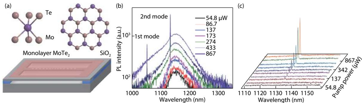
Fig. 5. (Color online) (a) Schematic of the proposed room temperature, suspended silicon nanobeam laser with a monolayer MoTe<sub>2</sub> on top. The corresponding lasing spectra of the nanobeam laser under different pump power levels (b) using a grating resolution: 150 g/mm (0.41 nm), and (c) using a grating resolution: 600 g/mm (0.09 nm).
