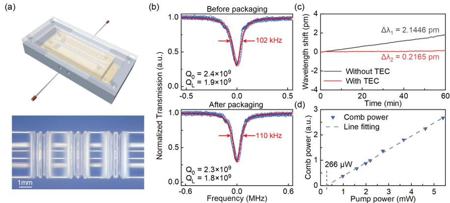
Fig. 1. (a) Top: schematic diagram of the packaged microrod resonator; bottom: optical imaging of the microrod resonator. (b) Measured greater than 2 billion  $Q$  of the microrod resonator before and after packaging. (c) The stability of the packaged microrod resonator over 1 hour without and with TEC. (d) Parametric oscillation power versus pump power showing an oscillation threshold of 266  $\mu$ W.
