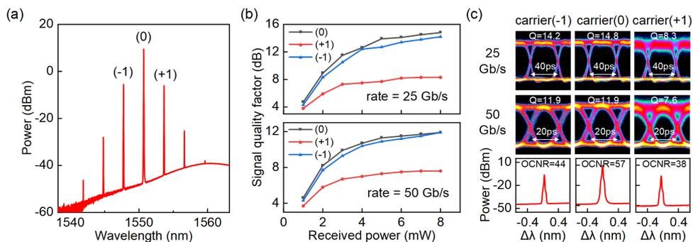
Fig. 2. (a) Spectrum of Kerr OFC generated in the packaged microrod resonator. (b) Measured signal quality factors as change of received power at different channel with the data rate of 25 Gb/s (top) and 50 Gb/s (bottom). (c) Eye diagrams and the corresponding OCNRs for each channel.
