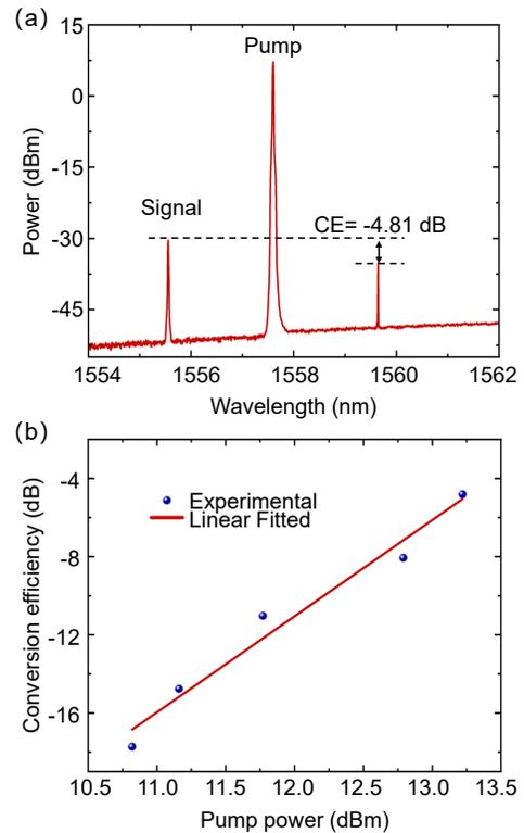
Fig. 2. (a) The measured FWM spectra in the packaged microrod resonator. (b) FWM-CE of the packaged microrod resonator. Horizontal axis is pump power while vertical axis is the CE.
