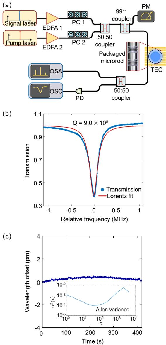
Fig. 1. (a) FWM-based wavelength conversion experimental setup. EDFA, Erbium-doped fiber amplifier; PC, fiber polarization controller; PD, photodetector; OSA, optical spectrum analyzer; OSC, oscilloscope; PM, power meter. (b) Transmission spectrum of the packaged microrod resonator. (c) Real time stability of the packaged microrod resonator. Inset: Allan variance of the system intrinsic noise.
