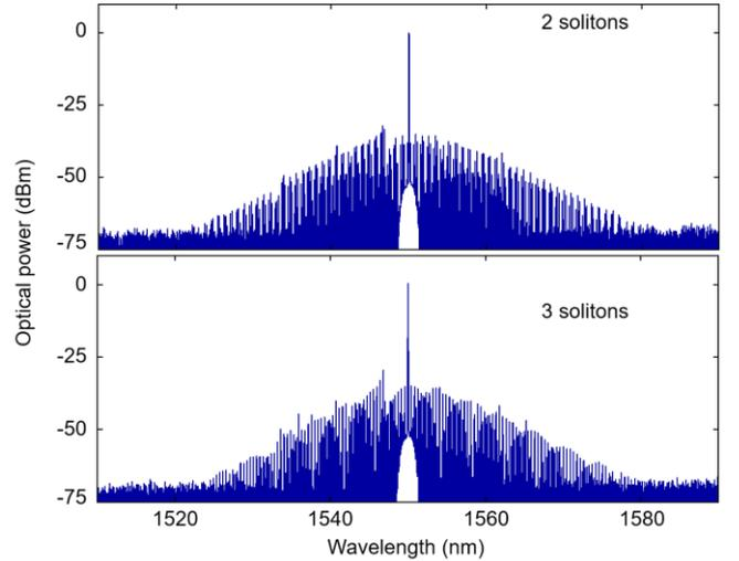
Fig. 3. Frequency comb spectra of selected soliton states with two and three solitons.
